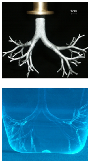
Fig. 2 Positive model of the human bronchial tree (top), silicone model with hollow branches used for measurements (bottom)
